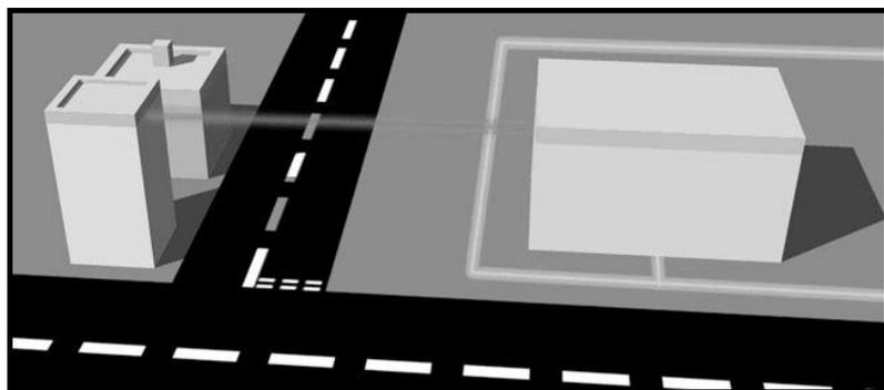
Two or more vehicles or buildings are connected by CableFree wireless products. Clear Line-of-Sight (LOS) for FSO or Near-Line-of-Sight (NLOS) for radio is required.
