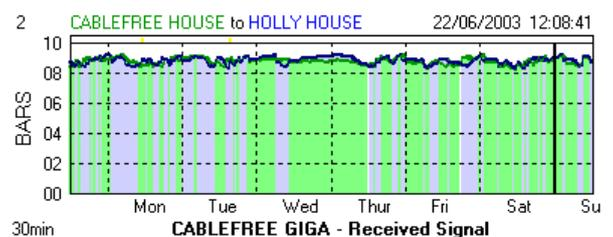
CableFree links without (top) and with (above) ATPC turned on. The received signal level varies greatly without ATPC, due to fog and rain storms. With the system switched on, TX power is adjusted to produce near constant power at the receiver, making a huge improvement to link performance, availability and BER
