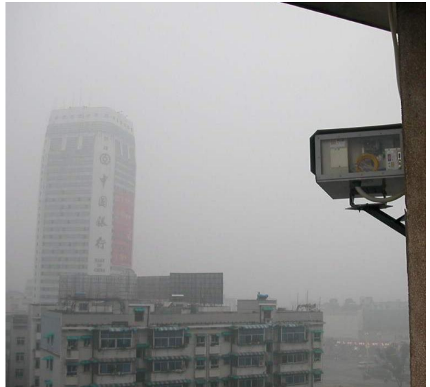
CableFree FSO deployed in Hunan Province, China. Industrial smog produces high attenuation which limits transmission distances to 1km. Sophisticated planning tools are used to predict link availability. CableFree UNITY solutions use diverse media (FSO+radio, FSO+MMW, MMW+Microwave) to extend range, capacity and availability by combining different wireless technologies
